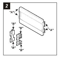
Cut and remove mounting tabs "A" from Radio Housing #1. Locate the v-cut on the back of each Mounting Bracket, cut along the v-cut and remove the back portion of each Bracket ("B"). (The tabs can be identified by the stamped letter on the back of each tab). Skip to the Installation Instructions for ALL VEHICLES on Page #3.
