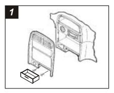
Disconnect the negative battery terminal to prevent an accidental short circuit. Remove the ashtray and (2) Phillips screws exposed in the ashtray cavity. Unclip the dash trim bezel and remove. Remove (4) Phillips screws securing the factory head unit and disconnect the wiring.
