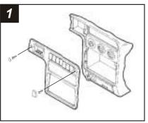
Disconnect the negative battery terminal to prevent an accidental short circuit. Pop off the plastic screw cover located to the left of the coin tray and remove (1) Phillips screw exposed. Using a small flat-blade screwdriver, pop out the dummy switch located in the far right position of the switch panel and remove (1) Phillips screw exposed. Unclip the dash trim bezel and remove. Remove (4) Phillips screws securing the factory head unit and disconnect the wiring.
