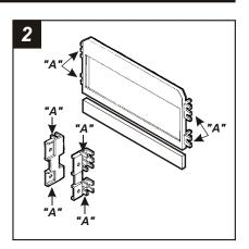
Cut and remove mounting tabs "A" from the *Mounting Brackets* and *Radio Housing #2*. (The tabs can be identified by the stamped letter on the back of each tab). Locate the scored line on the back of the Radio Housing and break away the bottom portion of the Housing as shown. *Skip to the Installation Instructions for ALL VEHICLES on Page #3*.
