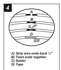
Locate the factory wiring harness in the dash. Metra recommends using the proper mating adaptor and making connections as shown. (Isolate and individually tape off the ends of any unused wires to prevent electrical short circuit).
