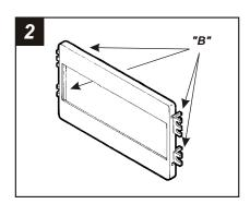
Cut and remove mounting tabs "B" from Radio Housing #1. (The tabs can be identified by the stamped letter on the back of each tab). Skip to the Installation Instructions for ALL VEHICLES on Page #3.
