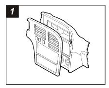
Disconnect the negative battery terminal to prevent an accidental short circuit. Remove (2) Phillips screws above the instrument cluster. Unclip the entire dash trim bezel and remove. Remove (4) screws securing the factory head unit and disconnect the wiring.
