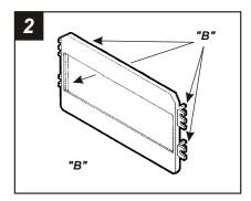
Cut and remove mounting tabs "B" from Radio Housing #2. (The tabs can be identified by the stamped letter on the back of each tab). Skip to the Installation Instructions for ALL VEHICLES on Page #3.
