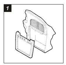
Disconnect the negative battery terminal to prevent an accidental short circuit. Unclip the radio trim bezel and remove. Remove (4) Phillips screws securing the factory head unit and disconnect the wiring.
