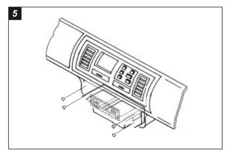
Insert the (4) Rubber Plugs into the Radio Housing over the mounted screw heads.
