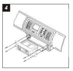
Re-connect the battery terminal and test the unit for proper operation. Mount the head unit/kit assembly to the sub-dash with (4) **Phillips Panhead Screws** supplied.
