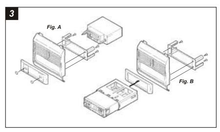
**2-SHAFT HEAD UNITS:** Align the radio opening in the **Radio Housing** with the radio opening in the radio trim bezel and mount the Housing to the back of the bezel with **(4) Phillips Panhead Screws** supplied. Place the desired **Faceplate** against the front of the bezel. Slide the aftermarket head unit through the assembly and secure with shaft nuts. (see Fig. A)
