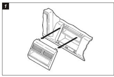
Disconnect the negative battery terminal to prevent an accidental short circuit. Pull out on the bottom of the radio trim bezel. Unhook the top corners of the bezel and remove.
