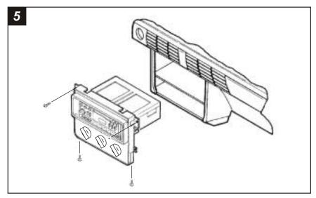
Re-connect the battery terminal and test the unit for proper operation. Mount the head unit/kit assembly to the sub-dash with (4) screws previoulsy removed in step #1.
