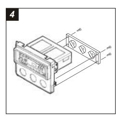
Mount the climate controls to the back of the *Replacement Bezel* with (4) screws previously removed in step #1.
