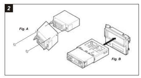
**2-SHAFT HEAD UNITS:** Slide the aftermarket head unit into the kit and secure with shaft nuts. (see Fig. A)
