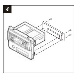
Mount the climate controls to the back of the *Replacement Bezel* with (4) screws previously removed in step #1.
