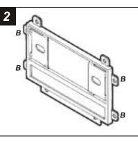
Disconnect the negative battery terminal to prevent an accidental short circuit. Unclip the dash trim bezel and remove. Remove (4) Phillips screws securing the factory head unit and disconnect the wiring. Cut and remove all mounting tabs on the **Radio Housing** EXCEPT tabs **"B"**. The mounting tabs cab be identified by the stamped letter on the back of each tab. *Skip* to the Installation Instructions for ALL VEHICLES on Page #3.
