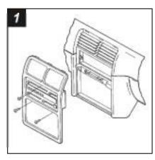
Disconnect the negative battery terminal to prevent an accidental short circuit. Remove the climate control knobs. Remove (1) Phillips screw above and (2) Phillips screws below the climate controls. Unclip the radio trim bezel. Remove (4) screws from the factory head unit. slide the unit out and disconnect the wiring.
