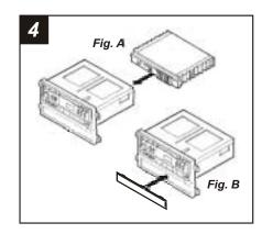
**IF AN EQUALIZER WILL BE INCLUDED :** Slide the aftermarket equalizer into the back of the **Radio Housing.** Using the hardware included with the equalizer, mount the unit to the kit. (see Fig. A)
