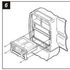
Re-connect the battery terminal and test the unit for proper operation. Slide (4) Speed Clips over the holes in the sub-dash mounting brackets and mount the head unit/kit assembly with (4) Phillips Pan-Head Screws supplied.
