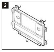
Cut and remove all mounting tabs on the Radio Housing EXCEPT tabs "A". The mounting tabs can be identified by the stamped letter on the back of each tab. Skip to the Installation Instructions for ALL VEHICLES on Page #3.
