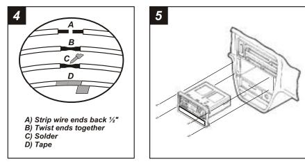
Locate the factory wiring harness in the dash. Metra recommends using the proper mating adaptor and making connections as shown. (Isolate and individually tape off the ends of any unused wires to prevent electrical short circuit). Re-connect the battery terminal and test the unit for proper operation. Mount the head unit/kit assembly to the sub-dash with (4) screws previously removed.
