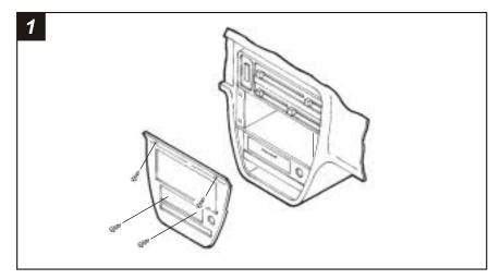
Disconnect the negative battery terminal to prevent an accidental short circuit. Remove the ashtray and (2) Phillips screws exposed. Remove (2) Phillips screws above the radio opening. Unclip the radio trim bezel and disconnect the cigarette lighter wiring. Remove (2) screws securing each side of the factory head unit and (1) screw from the rear support. Slide the unit out and disconnect the wiring.
