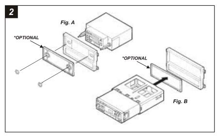
**<u>2-SHAFT HEAD UNITS:</u>** Slide the aftermarket head unit into the kit and secure with shaft nuts. (see Fig. A)
