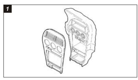
Disconnect the negative battery terminal to prevent an accidental short circuit. Remove the ashtray and (2) Phillips screws exposed. Remove the ashtray. Grasp the bottom edge of the dash trim bezel, pull out on the bezel and remove (it may be necessary to use a panel removal tool). Disconnect the hazard switch and cigarette lighter wiring and remove the panel. Remove (4) screws securing the factory head unit and disconnect the wiring.
