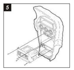
Re-connect the battery terminal and test the unit for proper operation. Mount the head unit/cupholder assembly to the sub-dash with (4) screws previously removed.
