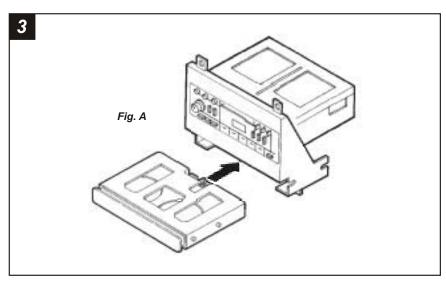
Remove the cupholder from the factory head unit assembly. Slide the cupholder into the bottom of the *Radio Housing* until the bosses on the sides of the cupholder engage the slots in the Housing. (see Fig. A)
