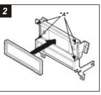
Locate the faceplate supplied with the aftermarket head unit. Place the faceplate into the recessed opening in the **Radio Housing.** If the faceplate fits easily into the opening with no interference, leave the Housing intact. If the faceplate does NOT fit easily into the opening, trim away the ribs located on the top and bottom of the opening ("A").
