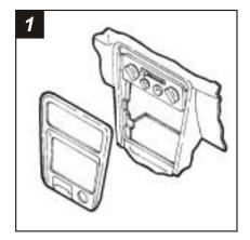
Disconnect the negative battery terminal to prevent an accidental short circuit. Remove the ashtray. Unclip the radio trim bezel and disconnect the wiring. Remove (4) Phillips screws securing the factory head unit/cupholder assembly, slide the assembly out and disconnect the wiring.
