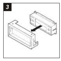
Slide the *Extension Housing* into the *Radio Housing* until the desired depth has been established.
