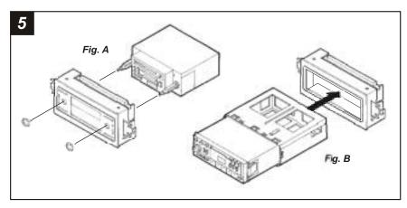
**2-SHAFT HEAD UNITS:** Slide the aftermarket head unit into the kit and secure with shaft nuts. (see Fig. A)
