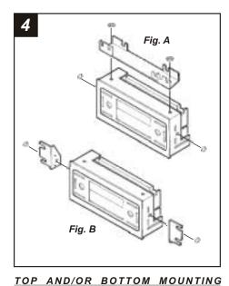
BRACKETS: Mount the Extension Housing to the Radio Housing with (2) Carriage Bolts and (2) Keps Nuts. Mount the bracket(s) to the housing assembly with Carriage Bolts and Keps Nuts supplied. (see Fig. A)
