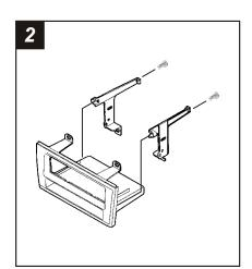
Secure the *Mounting Brackets* to the *Radio Housing* with (2) #8 x 3/8" *Phillips Truss-head Screws* supplied.
