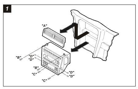
Disconnect the negative battery terminal to prevent an accidental short circuit. Unclip the a/c vent panel ("A") and remove (2) Phillips screws exposed at the top of the factory head unit ("B"). Remove (2) Phillips screws below the climate control pod ("C"). Slide the head unit/climate control pod assembly from the dash cavity and disconnect the wiring. Remove (4) Phillips screws securing the climate control pod to the factory brackets ("D") and remove the pod.
