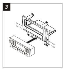
Slide the climate control pod into the *Radio Housing* and secure with (4) #8 x 3/8" *Phillips Pan-head Screws* supplied
