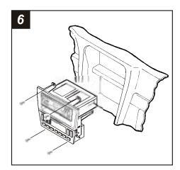
Re-connect the battery terminal and test the unit for proper operation. Mount the head unit/climate control pod assembly to the sub-dash with (4) Phillips screws previously removed in step #1. Replace the a/c vent panel.
