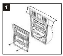
Disconnect the negative battery terminal to prevent an accidental short circuit. Open the ashtray and remove (2) Phillips screws securing the dash trim bezel. Remove (4) screws securing the factory head unit and disconnect the wiring.
