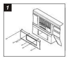
Disconnect the negative battery terminal to prevent an accidental short circuit. Remove (3) #8 Phillips screws from the bottom of the radio trim bezel. Unsnap the plastic strip located above the bezel and remove (3) Phillips screws exposed. Gently pull the instrument cluster trim bezel away from the dash and remove the radio trim bezel. Remove (3) hex-head screws securing the factory head unit and disconnect the wiring.
