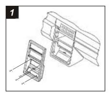
Disconnect the negative battery terminal to prevent an accidental short circuit. Remove (2) #8 Phillips screws below the radio opening. Open the ashtray and remove (2) #8 Phillips screws exposed (it is NOT necessary to remove the center screw). Unclip and remove the dash trim bezel. Remove (4) hex-head screws securing the factory head unit and disconnect the wiring.
