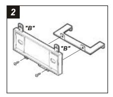
Cut and remove all mounting tabs on the *Radio Housing* EXCEPT tabs "B". The mounting tabs can be identified by the stamped letter on the back of each tab. Mount *Bracket #2* to the bottom of the Housing with (2) #8 x 1" *Phillips Screws* supplied. Skip to the Installation Instructions for ALL VEHICLES on Page #22.
