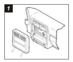
Disconnect the negative battery terminal to prevent an accidental short circuit. Remove (4) Phillips screws from the bottom of the dash trim bezel. Remove the bezel. Remove (2) screws securing the factory head unit and disconnect the wiring.
