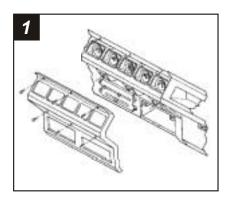
Disconnect the negative battery terminal to prevent an accidental short circuit. Remove (6) Phillips screws from the face of the dash trim bezel. Remove the bezel. Remove (2) screws securing the factory head unit and disconnect the wiring.
