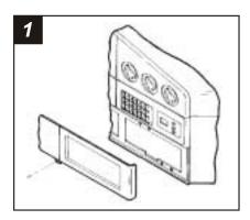
Disconnect the negative battery terminal to prevent an accidental short circuit. Remove (1) 7mm hex-head screw from the bottom of the radio trim bezel. Gently unclip the bezel and disconnect the antenna switch power lead. Remove (4) screws securing the factory head unit and disconnect the wiring.
