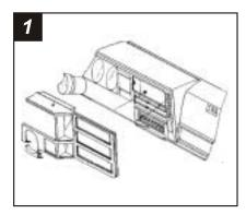
Disconnect the negative battery terminal to prevent an accidental short circuit. Unsnap the steering column trim panel and remove. Remove (4) screws from the dash trim bezel and remove the bezel. Remove (2) screws securing the factory head unit and disconnect the wiring.
