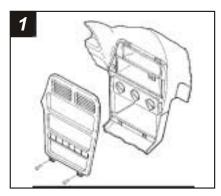
Disconnect the negative battery terminal to prevent an accidental short circuit. Remove (2) screws from the base of the dash trim bezel. Unclip and remove the bezel. Using Metra's 86-5618, pull the factory head unit from the dash and disconnect the wiring.
