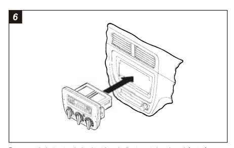
Re-connect the battery terminal and test the unit, climate controls and rear defroster for proper operation. Snap the *Integrated Mounting Kit* assembly into the sub-dash.
