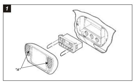
Disconnect the negative battery terminal to prevent an accidental short circuit. Place your index fingers on the inner edges of the a/c vents (shown above) and push inward. Grasp the exposed lip of each vent opening ("A") and pull out on the radio trim bezel. Remove the dash trim bezel. (The airbag wiring does NOT need to be disconnected). Using Metra's 86-5618 or AW-FDRT, pull the factory head unit from the dash and disconnect the wiring.
