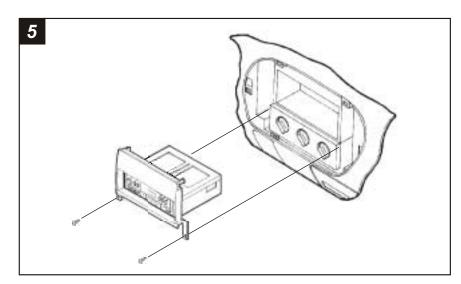
Re-connect the battery terminal and test the unit for proper operation. Remove the top (2) Phillips screws securing the climate control cluster to the sub-dash. Slide the head unit/kit assembly into the dash cavity (be sure the *Rear Support Bracket* engages the support shelf in the dash). Mount the bottom legs of the kit to the same holes in the climate control cluster with the (2) Phillips screws previously removed.
