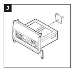
Mount the **Rear Support Bracket** to the back of the head unit with the necessary hardware.
