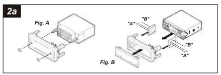
2-SHAFT HEAD UNITS: Attach the 2-Shaft Faceplate and Shaft Masks to the Radio Housing. Slide the aftermarket head unit into the kit and secure with shaft nuts. (see Fig. A)
