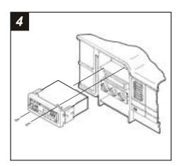
Re-connect the battery terminal and test the unit for proper operation. Mount the head unit/kit assembly to the sub-dash with those screws previously removed in the dash disassembly.
