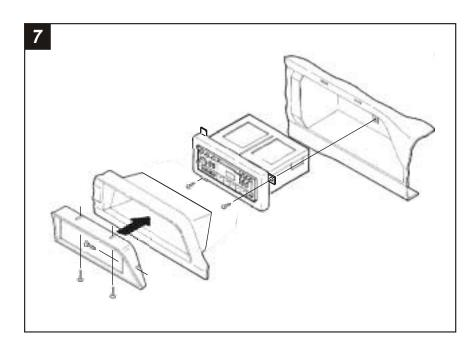
Re-connect the battery terminal and test the unit for proper operation. Mount the head unit/kit assembly to the sub-dash with (2) screws. Place the Faceplate into the dash trim bezel and mount with (3) 3/8" Phillips screws supplied.
