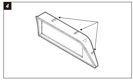
Locate the recessed slots on the top of the *Faceplate* and drill (1) 3/16" hole into each slot.
