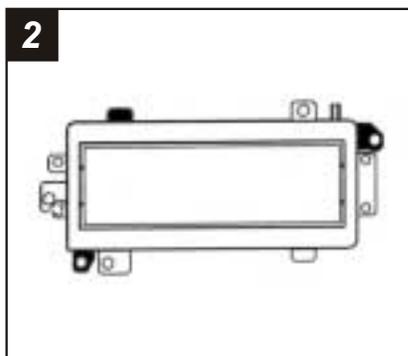
Cut and remove all mounting tabs on the **Radio Housing** EXCEPT the shaded tabs. Skip to the Installation Instructions for ALL VEHICLES on Page #20.
