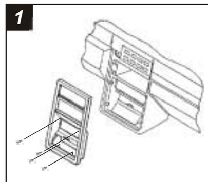
Disconnect the negative battery terminal to prevent an accidental short circuit. Remove (2) #8 Phillips screws below the radio opening. Open the ashtray and remove (2) #8 Phillips screws (it is NOT necessary to remove the center screw). Unclip the dash trim bezel and remove. Remove (4) hex-head screws securing the factory head unit and disconnect the wiring.
