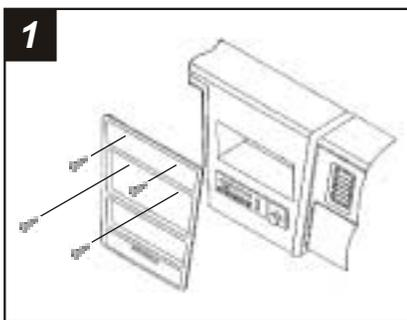
Disconnect the negative battery terminal to prevent an accidental short circuit. Remove (2) Phillips screws above the radio opening. Remove (2) Phillips screws above the climate controls. Unclip the dash trim bezel and remove. Remove (2) 3/8" hex-head screws securing the factory head unit and disconnect the wiring.
