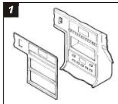
Disconnect the negative battery terminal to prevent an accidental short circuit. Pry out on the dash trim bezel and remove. Remove (4) 5mm hex-head sheet metal screws securing the factory head unit and disconnect the wiring.
