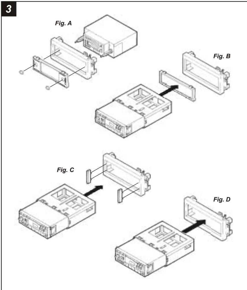
**2-SHAFT HEAD UNITS:** Snap the **Faceplate** into the **Radio Housing**. Slide the aftermarket head unit into the kit and secure with shaft nuts. (see Fig. A)
