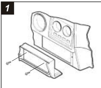
Disconnect the negative battery terminal to prevent an accidental short circuit. Remove (4) Phillips screws from the bottom edge of the radio trim bezel. Remove (2) Phillips screws above the radio opening. Unscrew the retainer ring securing the remote mirror control and remove the bezel. Remove (2) 3/8" hex-head screws securing the factory head unit and disconnect the wiring.
