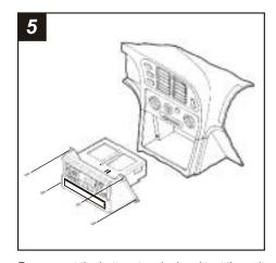
Re-connect the battery terminal and test the unit for proper operation. Mount the head unit/kit assembly to the sub-dash with (4) Phillips screws previously removed in step #1.
