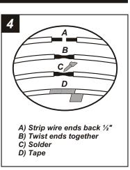
Locate the factory wiring harness in the dash. Metra recommends using the proper mating adaptor and making connections as shown. (Isolate and individually tape off the ends of any unused wires to prevent electrical short circuit).
