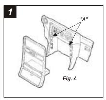
Disconnect the negative battery terminal to prevent an accidental short circuit. Unclip the gear shifter trim panel and remove (1) screw exposed. Unclip the dash trim bezel and remove. Remove (4) Phillips screws securing the factory head unit and disconnect the wiring. Cut and remove tabs "A" located in the top corners of the dash cavity.
