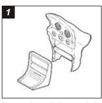
Disconnect the negative battery terminal to prevent an accidental short circuit. Remove (4) Phillips screws securing the center console. Pry out on the front edge of the console and unclip the radio trim bezel. Remove (2) Phillips screws securing the factory pocket and remove. Remove (4) Phillips screws securing the factory head unit and disconnect the wiring.
