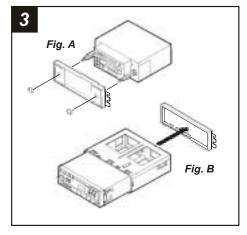
**<u>2-SHAFT HEAD UNITS:</u>** Slide the aftermarket head unit into the **Radio Housing** and secure with shaft nuts. (see Fig. A).
