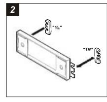
Attach **Spacer 1L** to the left mounting tab of the **Radio Housing** and **Spacer 1R** to the right mounting tab of the **Radio Housing** as shown. Skip to the Installation Instructions for ALL VEHICLES on Page #3.
