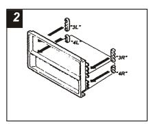
Attach Spacer 3L and 4L to the left mounting tabs of the Radio Housing and Spacer 3R and 4R to the right mounting tabs of the Radio Housing as shown.
