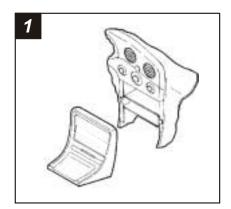
Disconnect the negative battery terminal to prevent an accidental short circuit. Remove (4) Phillips screws securing the center console. Pry out on the front edge of the console and unclip the radio trim bezel. Remove (2) Phillips screws securing the factory pocket and remove. Remove (4) Phillips screws securing the factory head unit and disconnect the wiring.
