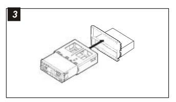
Slide the DIN cage into the kit and secure by bending the metal locking tabs down. Slide the aftermarket head unit into the cage until secure.
