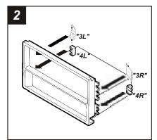
Attach **Spacer 3L** and **4L** to the left mounting tabs of the **Radio Housing** and **Spacer 3R** and **4R** to the right mounting tabs of the **Radio Housing** as shown. Skip to the Installation Instructions for ALL VEHICLES on Page #3.
