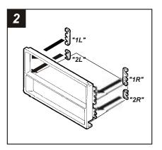
Attach **Spacer 1L** and **2L** to the left mounting tabs of the **Radio Housing** and **Spacer 1R** and **2R** to the right mounting tabs of the **Radio Housing** as shown. Skip to the Installation Instructions for ALL VEHICLES on Page #3.
