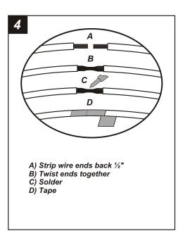
Locate the factory wiring harness in the dash. Metra recommends using the proper mating adaptor and making connections as shown. (Isolate and individually tape off the ends of any unused wires to prevent electrical short circuit).
