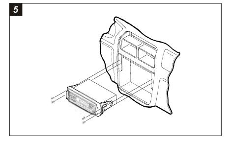
Re-connect the battery terminal and test the unit for proper operation. Mount the head unit/kit assembly to the sub-dash with (4) Phillips screws previously removed in step #1.
