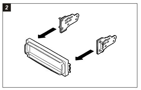
Snap the ISO Brackets over the mounting tabs on the Radio Housing.
