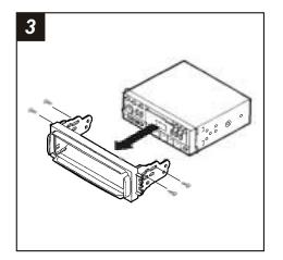
Slide the head unit into the *Radio Housing*, align the holes in the head unit with the holes in the Housing and mount the unit with the screws supplied with the unit.
