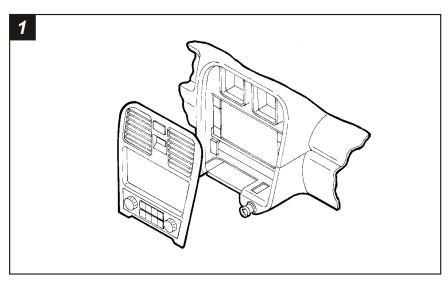
Disconnect the negative battery terminal to prevent an accidental short circuit. Unclip the dash trim bezel. Disconnect the clock and climate control wiring and remove the bezel. Remove (4) Phillips screws securing the factory head unit and disconnect the wiring.
