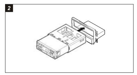
Slide the DIN cage into the *Radio Housing* and secure by bending the metal locking tabs down. Slide the aftermarket head unit into the cage until secure.
