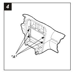
Locate the (4) mounting positions in the sub-dash ("A").
