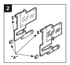
Using the raised lines as a guide, cut and remove the ends of each *Mounting Bracket* ("A").
