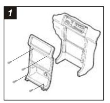
Disconnect the negative battery terminal to prevent an accidental short circuit. Unclip the gear shifter trim bezel and remove (2) Phillips screws exposed. Remove (2) Phillips screws above the radio opening. Unclip the radio trim bezel. Remove (4) Phillips screws from the factory head unit and disconnect the wiring.
