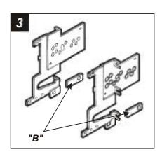
Using the corner of each mounting tab as a guide, cut and remove the ends of the cupholder mounts from the **Mounting Brackets** ("B").
