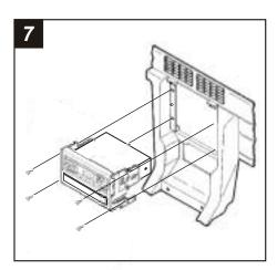
Re-connect the battery terminal and test the unit for proper operation. Mount the head unit/kit assembly to the sub-dash with (4) Phillips screws removed in step #1.
