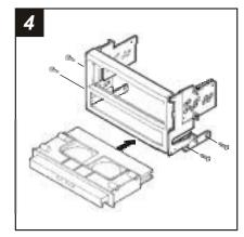
Remove (4) screws securing the cupholder to the factory head unit assembly and remove. Slide the cupholder into the bottom of the *Radio Housing* and mount with the same (4) screws. Skip to the Installation Instructions for ALL VEHICLES on Page #3.
