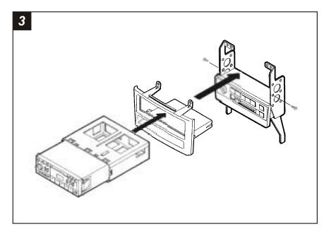
Mount the *Radio Housing* to the factory brackets with (2) #8 x ½" *Phillips Truss-Head Screws* supplied. Slide the DIN cage into the Radio Housing and secure by bending the metal locking tabs down. Slide the aftermarket head unit into the cage until secure.
