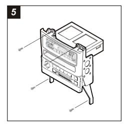
Re-connect the battery terminal and test the unit for proper operation. Mount the factory bracket assembly to the sub-dash with (4) Phillips screws previously removed in step #1.
