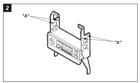
Using a hammer, flatten the protruding screw holes ("A") on the factory brackets.
