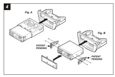
**DIN HEAD UNITS:** Slide the DIN cage into the kit and secure by bending the metal locking tabs down. Slide the aftermarket head unit into the cage until secure. (see Fig. A) **ISO HEAD UNITS:** Secure the **ISO Brackets** to the sides of the aftermarket head unit with the screws supplied with the unit. Slide the head unit assembly into the **Radio Housing** until the side clips engage and attach the **ISO Trimring** over the mounted head unit. (see Fig. B).
