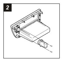
Mount the hazard switch to the back of the *Radio Housing* with (2) Phillips screws previously removed in step #1.
