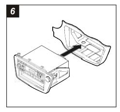
Re-connect the battery terminal and test the unit for proper operation. Re-connect the hazard switch plug and snap the head unit/kit assembly into the sub-dash.
