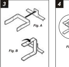
Insert the **Radio Support** into the **Mounting Bracket**. (see Fig. A). Turn the Radio Support to lock into place. (see Fig. B)
