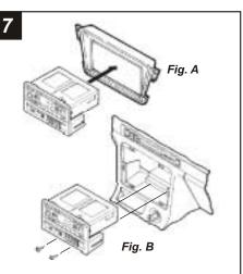
ACCORD 1990-93, INTEGRA, ODYSSEY, OASIS: Re-connect the battery terminal and test the unit for proper operation. Snap the head unit/kit assembly into the sub-dash.
