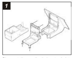
Disconnect the negative battery terminal to prevent an accidental short circuit. Remove the ashtray and (1) ¾" #8 Phillips screw exposed. Open the storage compartment and remove (2) #8 Phillips screws exposed. Remove the cupholder tray and (3) #8 Phillips screws inside. Lift the center console out and remove (2) Phillips screws exposed at the base of the dash trim bezel. Unclip the bezel and remove. Remove (2) hex-head screws securing the factory head unit and disconnect the wiring.
