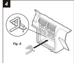
Insert the *Radio Support* into the *Mounting Bracket.* (see *Fig. A*). Turn the Radio Support to lock into place. (see *Fig. B*)
