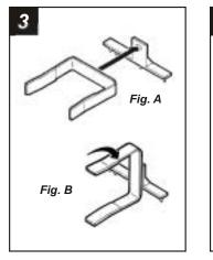
Insert the **Radio Support** into the **Mounting Bracket**. (see Fig. A). Turn the Radio Support to lock into place. (see Fig. B) Fig. A
