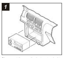
Disconnect the negative battery terminal to prevent an accidental short circuit. Remove (4) screws from the lower portion of the center console. Remove the gear shifter knob and lift the console out. Remove the ashtray and ashtray bracket. Remove (2) screws from the bottom of the head unit support, slide the unit out and disconnect the wiring.
