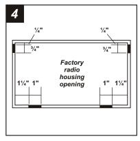
Modify the factory radio housing by trimming the *shaded* portions of the housing lip. *Skip to the Installation Instructions for ALL VEHICLES on Page* #11.
