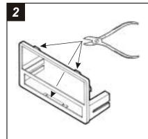
Cut and remove the *TOP* clips and *BOTTOM* tab from the *Radio Housing*.
