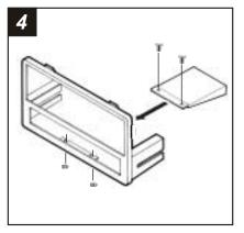
Mount the **Rear Support Bracket** to the bottom tab on the **Radio Housing** with (2) **Carriage Bolts** and (2) **Nuts.** Skip to the Installation Instructions for ALL VEHICLES on Page #11.
