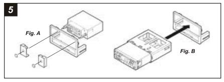
**<u>2-SHAFT HEAD UNITS</u>**: Snap the **Shaft Supports** into the **Radio Housing**. Slide the aftermarket head unit into the kit and secure with shaft nuts. (see Fig. A)
