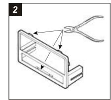
Cut and remove the *TOP* clips and *BOTTOM* tab from the *Radio Housing*.
