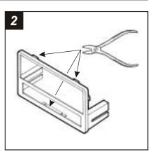
Cut and remove the *TOP* clips and *BOTTOM* tab from the *Radio Housing*.
