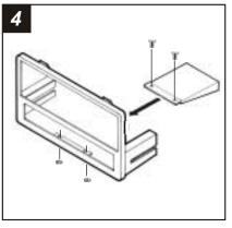
Mount the **Rear Support Bracket** to the bottom tab on the **Radio Housing** with (2) **Carriage Bolts** and (2) **Keps Nuts.** Skip to the Installation Instructions for ALL VEHICLES on Page #11.
