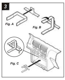
Insert the *Radio Support* into the *Mounting Bracket.* (see *Fig. A*). Turn the Radio Support to lock into place. (see *Fig. B*). Mount the assembly to the sub-dash mounting plate with (2) *Pal Nuts* supplied. (see *Fig. C*)
