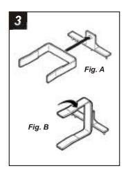
Insert the *Radio Support* into the *Mounting Bracket.* (see Fig. A). Turn the Radio Support to lock into place. (see Fig. B)
