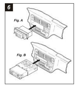
**2-SHAFT HEAD UNITS:** Re-connect the battery terminal and test the unit for proper operation. Snap the head unit/kit assembly into the subdash. Be sure the unit engages the **Radio Support** in the dash. (see Fig. A)
