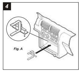
Mount the assembly to the factory mounting plate in the sub-dash with (2) Pal Nuts supplied. (see Fig. A)
