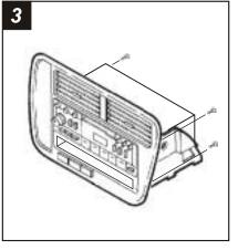
Remove (4) Phillips screws securing the head unit assembly to the back of the dash trim bezel.
