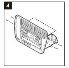
Remove (4) Phillips screws securing the factory brackets to the head unit assembly and slide the assembly out the front of the dash trim bezel.
