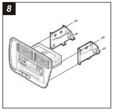
Mount the factory brackets to the back of the dash trim bezel with (4) Phillips screws previously removed in step #3.
