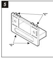
Cut and remove all mounting clips on the *Radio Housing* EXCEPT clips "*C*". The mounting clips can be identified by the stamped letter on each clip.
