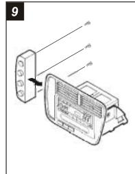
Mount the climate control pod to the dash trim bezel with (3) screws previously removed in step #2.
