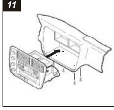
Re-connect the battery terminal and test the unit for proper operation. Slide the head unit/kit assembly into the sub-dash and mount with (4) Phillips screws previously removed in step #1.
