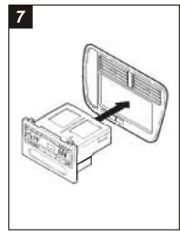
**<u>2-SHAFT HEAD UNITS:</u>** Slide the aftermarket head unit into the **Radio Housing** and secure with shaft nuts. (see Fig. A)
