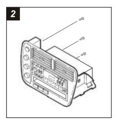
Remove (3) screws securing the climate control pod to the dash trim bezel and remove the pod.
