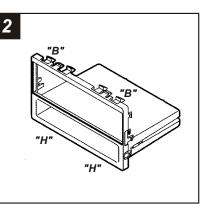
Cut and remove the all mounting clips on the *Radio Housing* EXCEPT clips "*B*" and "*H*". (The clips can be identified by the stamped letter near each clip). *Skip to step #3b on Page 11.*
