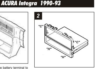
Cut and remove the all mounting clips on the *Radio Housing* EXCEPT clips "*C*" and "*H*". (The clips can be identified by the stamped letter near each clip). *Skip to step #3b on Page 11.*
