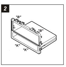
Cut and remove the all mounting clips on the *Radio Housing* EXCEPT clips "*B*" and "*K*". (The clips can be identified by the stamped letter near each clip). *Skip to step #3b on Page 11.*
