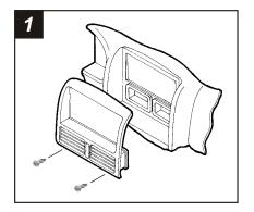
Disconnect the negative battery terminal to prevent an accidental short circuit. Remove (2) Phillips screws from the bottom edge of the radio trim bezel. Unclip the trim bezel and remove. Remove (4) Phillips screws securing the factory head unit and disconnect the wiring.
