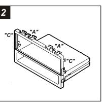
Cut and remove the all mounting clips on the *Radio Housing* EXCEPT clips "A" and "C". (The clips can be identified by the stamped letter near each clip). *Skip to step #3b on Page 11.*
