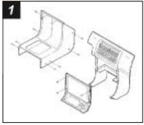
Disconnect the negative battery terminal to prevent an accidental short circuit. Remove (2) screws from the top of the console trim bezel. Slide the front seats back and remove (4) Phillips screws from each side of the bezel. Pull up on the console trim bezel and remove. Using an angled screwdriver, remove (2) screws securing the gear shifter bracket to the bezel. Remove (4) screws from the radio trim bezel, remove the factory head unit assembly and disconnect the wiring.
