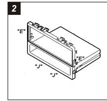
Cut and remove the all mounting clips on the *Radio Housing* EXCEPT clips *"E"* and *"J"*. (The clips can be identified by the stamped letter near each clip). *Skip to step #3b on Page 11*.
