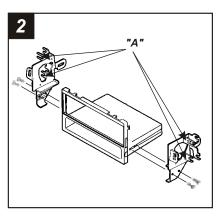
Cut and remove the mounting clips from the **Radio Housing.** Locate tabs "A" on the **Mounting Brackets** for mounting, cut and remove tabs "B". (The tabs can be identified by the stamped letter near each tab). Secure the Brackets to the Housing with (4) **#8 x 3/8" Phillips Pan-head Screws.** Skip to step #3b on Page 11.
