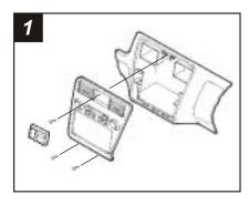
Disconnect the negative battery terminal to prevent an accidental short circuit. Unsnap the clock panel, disconnect the wiring and remove. Remove (1) Phillips screw exposed in the clock cavity. Remove (2) Phillips screws below the factory head unit. Unclip the radio trim bezel and disconnect the wiring. Remove (4) Phillips screws securing the factory head unit assembly and disconnect the wiring. Remove (2) screws securing the factory pocket to the assembly.
