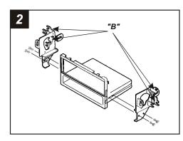
Cut and remove the mounting clips from the **Radio Housing.** Locate tabs **"B"** on the **Mounting Brackets** for mounting, cut and remove tabs **"A"**. (The tabs can be identified by the stamped letter near each tab). Secure the Brackets to the Housing with (4) #8 x 3/8" Phillips Pan-head Screws. Skip to step #3b on Page 11.
