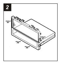
Cut and remove the all mounting clips on the **Radio Housing** EXCEPT clips **"D"** and **"H"**. (The clips can be identified by the stamped letter near each clip). *Skip to step #3b on Page 11*.
