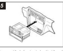
Re-connect the battery terminal and test the unit for proper operation. Slide the head unit/kit assembly into the sub-dash or trim bezel (depending on the vehicle) and secure by reversing the steps in the dash disassembly. ACCORD 1994-97 and CL 1997-99: Mount the Rear Support Bracket to the rear support provision with (2) bolts previously removed in the dash disassembly.
