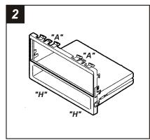
Cut and remove the all mounting clips on the *Radio Housing* EXCEPT clips "*A*" and "*H*". (The clips can be identified by the stamped letter near each clip). *Skip to step #3b on Page 11.*
