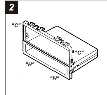
Cut and remove the all mounting clips on the *Radio Housing* EXCEPT clips *"C"* and *"H"*. (The clips can be identified by the stamped letter near each clip). *Skip to step #3b on Page 11*.
