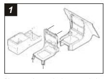
Disconnect the negative battery terminal to prevent an accidental short circuit. Remove the ashtray and (1) ¼" #8 Phillips screw exposed. Open the storage compartment and remove (2) #8 Phillips screws exposed. Remove the cupholder tray and (3) #8 Phillips screws inside. Lift the center console out and remove (2) Phillips screws exposed at the base of the dash trim bezel. Unclip the bezel and remove. Remove (2) hex-head screws securing the factory head unit and disconnect the wiring.
