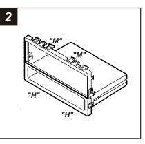
Cut and remove the all mounting clips on the *Radio Housing* EXCEPT clips *"M"* and *"H"*. (The clips can be identified by the stamped letter near each clip). *Skip to step #3b on Page 11.*
