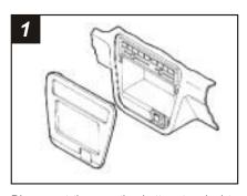
Disconnect the negative battery terminal to prevent an accidental short circuit. Using a panel removal tool, unclip the radio trim bezel and remove (some force may be required). Remove (4) Phillips screws securing the factory head unit/bracket housing assembly and disconnect the wiring. Remove (4) Phillips screws securing the factory head unit to the bracket housing and remove.
