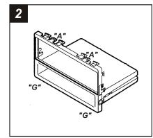
Cut and remove the all mounting clips on the *Radio Housing* EXCEPT clips "*A*" and "*G*". (The clips can be identified by the stamped letter near each clip). *Skip to step #3b on Page 11.*
