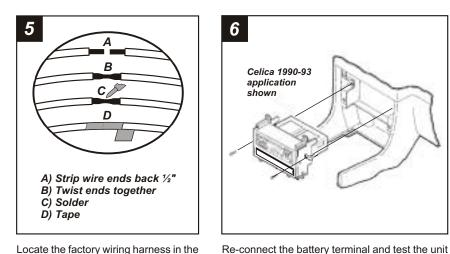
Locate the factory wiring harness in the dash. Metra recommends using the proper mating adaptor and making connections as shown. (Isolate and individually tape off the ends of any unused wires to prevent electrical short circuit).
