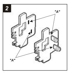
Slide Mounting Tabs #8 into slots "A" on Bracket Set #12. The Mounting Tabs, Brackets and Bracket slots can be identified by the stamped letter on each component. Skip to the Installation Instructions for ALL VEHICLES on Page #10.
