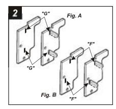
2DR/3DR MODELS: Slide Mounting Tabs #3 into slots "G" on Bracket Set #1. (see Fig. A).
