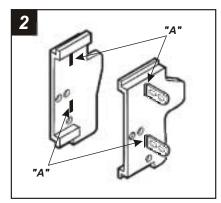
Slide *Mounting Tabs #3* into slots *"A"* on *Bracket Set #2.* The Mounting Tabs, Brackets and Bracket slots can be identified by the stamped letter on each component. *Skip to the Installation Instructions for ALL VEHICLES on Page #10.*
