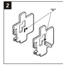
Slide *Mounting Tabs* #3 into slots "D" on *Bracket Set #12.* The Mounting Tabs, Brackets and Bracket slots can be identified by the stamped letter on each component. *Skip to the Installation Instructions for ALL VEHICLES on Page #10.*
