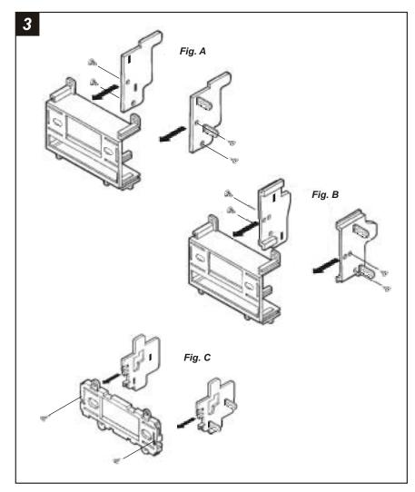
CELICA 1990-93, COROLLA (sport coupe/liftback) 1982-83, COROLLA (sedan/wagonlower dash) 1988-92, COROLLA 1984-87, LANDCRUISER 1988-92, MR2 1987-90, <u>PICKUP 1984-88, CRESSIDA, 4RUNNER:</u> Mount Bracket Set #1 to Radio Housing #1 with (4) Phillips Pan-head Screws supplied. (see Fig. A)
