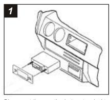
Disconnect the negative battery terminal to prevent an accidental short circuit. Remove (4) Phillips screws securing the factory head unit and disconnect the wiring.
