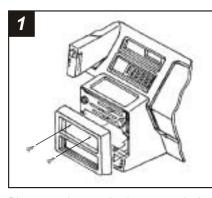
Disconnect the negative battery terminal to prevent an accidental short circuit. Remove (2) screws from the top of the dash trim bezel and remove the bezel. Remove (4) screws from the factory head unit (or coin tray dummy panel) and disconnect the wiring.
