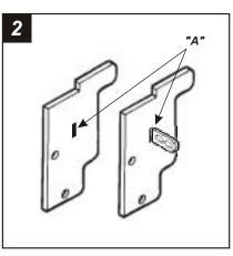
Slide *Mounting Tabs* #3 into slots "A" on *Bracket Set #1.* The Mounting Tabs, Brackets and Bracket slots can be identified by the stamped letter on each component. *Skip to the Installation Instructions for ALL VEHICLES on Page #10.*
