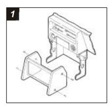
Disconnect the negative battery terminal to prevent an accidental short circuit. Remove (2) Phillips screws from each side of the radio trim bezel. Remove the bezel. Remove (4) screws securing the factory head unit and disconnect the wiring.
