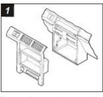
Disconnect the negative battery terminal to prevent an accidental short circuit. Remove (1) screw to the right of the ignition switch. Remove (1) screw above the left speaker. Unclip the dash trim bezel (some force may be required). Remove the screws securing the factory head unit and disconnect the wiring.
