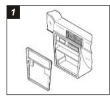
Disconnect the negative battery terminal to prevent an accidental short circuit. Unclip the climate control trim panel and remove (2) screws exposed. Remove (2) screws above the radio opening. Unclip the dash trim bezel, disconnect the wiring and remove the bezel. Remove (4) screws securing the factory head unit and disconnect the wiring.
