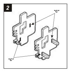
Slide *Mounting Tabs #3* into slots "C" on *Bracket Set #12.* The Mounting Tabs, Brackets and Bracket slots can be identified by the stamped letter on each component. *Skip to the Installation Instructions for ALL VEHICLES on Page #10.*
