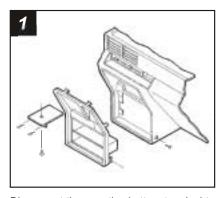
Disconnect the negative battery terminal to prevent an accidental short circuit. Remove the ashtray and (3) screws from the ashtray bracket. Remove (1) screw from each side of the dash console and unclip the dash trim bezel. Remove the screws securing the factory head unit and disconnect the wiring.
