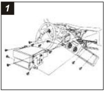
Disconnect the negative battery terminal to prevent an accidental short circuit. Remove (3) screws from the lower edge of the climate control panel. Remove (8) screws from the perimeter of the dash trim bezel. Pull out on the lower edge of the bezel and remove. Remove the screws securing the factory head unit and disconnect the wiring.
