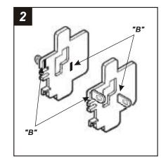
Slide *Mounting Tabs #3* and *#8* into slots "B" on Bracket Set #12. The Mounting Tabs. Brackets and Bracket slots can be identified by the stamped letter on each component. Skip to the Installation Instructions for ALL VEHICLES on Page #10.
