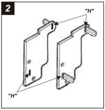
Slide *Mounting Tabs #3* into slots "H" on Bracket Set #1. The Mounting Tabs, Brackets and Bracket slots can be identified by the stamped letter on each component. Skip to the Installation Instructions for ALL VEHICLES on Page #10.
