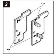
Slide **Mounting Tabs #3** into slots **"J"** and **"I"** on **Bracket Set #1.** The Mounting Tabs, Brackets and Bracket slots can be identified by the stamped letter on each component. *Skip to the Installation Instructions for ALL* VEHICLES on Page #10.
