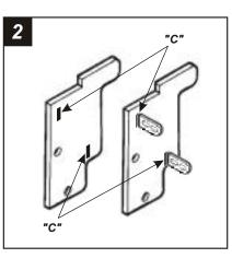
Slide Mounting Tabs #3 into slots "C" on Bracket Set #1. The Mounting Tabs, Brackets and Bracket slots can be identified by the stamped letter on each component. Skip to the Installation Instructions for ALL VEHICLES on Page #10.
