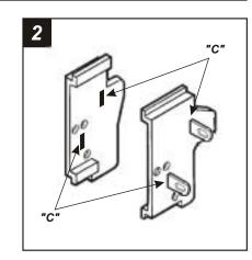
Slide *Mounting Tabs #8* into slots *"C"* on *Bracket Set #2.* The Mounting Tabs, Brackets and Bracket slots can be identified by the stamped letter on each component. *Skip to the Installation Instructions for ALL VEHICLES on Page #10.*
