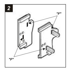
Slide *Mounting Tabs* #3 into slots "*F*" on *Bracket Set* #2. The Mounting Tabs, Brackets and Bracket slots can be identified by the stamped letter on each component. *Skip to the Installation Instructions for ALL VEHICLES on Page* #10.
