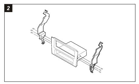
Mount the Mounting Brackets to the Radio Housing with (6) Phillips Screws supplied.
