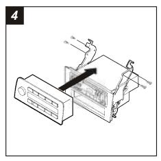
Position the factory climate control module above the *Radio Housing* and secure to the *Mounting Brackets* with (4) Phillips screws previously removed in step #1.
