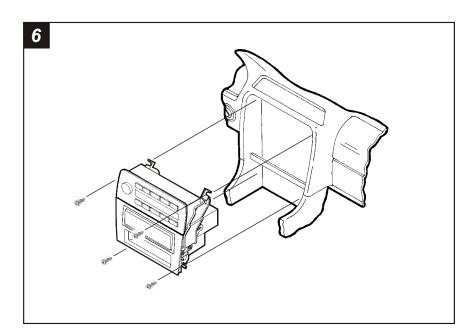
Re-connect the battery terminal and test the unit for proper operation. Mount the head unit/kit assembly to the sub-dash with (4) Phillips screws previously removed in step #1.
