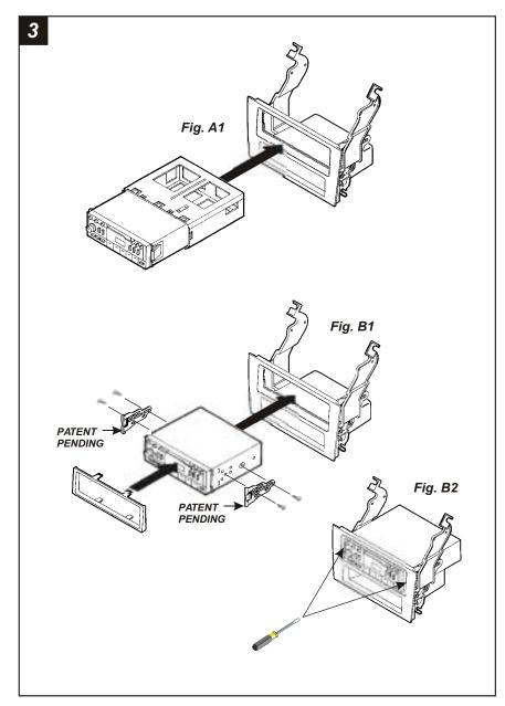
DIN HEAD UNITS: Slide the DIN cage into the Radio Housing and secure by bending the metal locking tabs down. Slide the aftermarket head unit into the cage and secure. (see Fig. A1)
