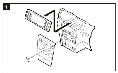
Disconnect the negative battery terminal to prevent an accidental short circuit. Unsnap the gear shifter trim bezel and remove. Remove the center climate control knob and (1) Phillips screw exposed. Unclip the climate control bezel/pocket assembly and remove. Remove (4) 10 mm bolts from the bottom of the factory head unit. Remove the factory head unit/trim bezel assembly and disconnect the wiring. Unclip the bezel from the head unit and remove the unit.
