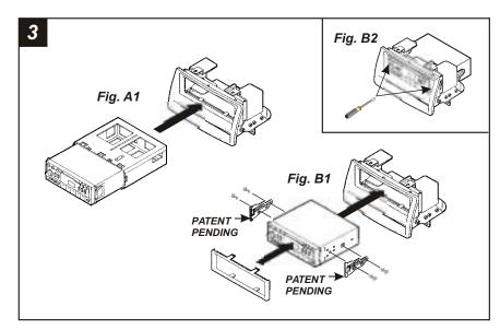
**<u>DIN HEAD UNITS:</u>** Slide the DIN cage into the **Radio Housing** and secure by bending the metal locking tabs down. Slide the aftermarket head unit into the cage and secure. (see Fig. A1)
