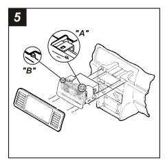
Re-connect the battery terminal and test the unit for proper operation. Snap the factory head unit trim bezel over the kit by engaging the (4) bracket tabs ("A") and (3) Housing bosses ("B") to the back of the bezel. Slide the assembly into the sub-dash and mount with (4) 10 mm bolts previously removed in step #1. Reassemble the dash.
