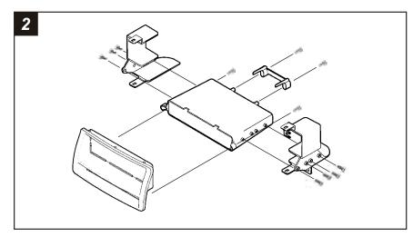
Attach the **Pocket** to the back of the **Radio Housing** (by holding the Housing upside-down, inserting the right edge of the Pocket into place and pushing the rest of the Pocket onto the lip) and mount with **(2)** #8 x 3/8" **Phillips Pan-head Screws** supplied. Secure the **Mounting Brackets** to the Pocket with **(8)** #6 x ½" **Phillip Flat-head Screws** supplied. Mount the **Rear Support Bracket** to the back of the Pocket with **(2)** #8 x 3/8" **Phillips Pan-head Screws** supplied.
