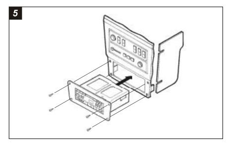
Re-connect the battery terminal and test the unit for proper operation. Mount the head unit/kit assembly to the sub-dash with (4) screws previously removed.
