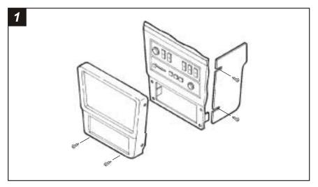
Disconnect the negative battery terminal to prevent an accidental short circuit. Remove (1) Phillips screw and (1) plastic twist-lock screw securing each side panel to the lower dash console. Remove (2) Phillips screws from the base of the radio trim bezel and remove the bezel. Remove (4) screws securing the factory pocket to the sub-dash and remove the pocket.
