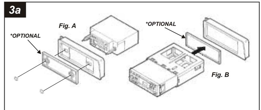
**200 SERIES (UPPER DASH):** For 2-Shaft head units, attach the **Spacer\*** to the **Radio Housing**. Slide the aftermarket head unit into the kit and secure with shaft nuts. (see Fig. A). For DIN head units, cut and remove the shaft supports from the **Spacer\*** and **Radio Housing**. Slide the DIN cage into the kit and secure by bending the metal locking tabs down. Slide the aftermarket head unit into the cage until secure. (see Fig. B)
