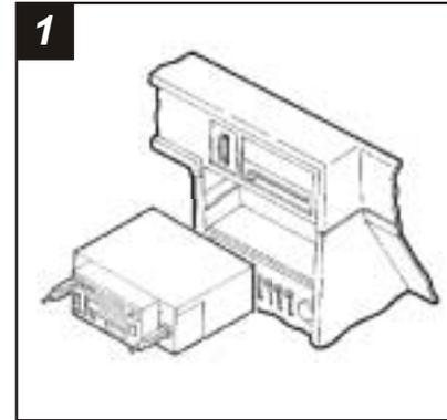
Disconnect the negative battery terminal to prevent an accidental short circuit. Remove (3) screws from the steering column inspection panel and lower the panel. Remove the factory radio knobs and shaft nuts. Insert a flat-blade screwdriver into the shaft wells and push in on the side springs. Pull the factory radio out and disconnect the wiring.
