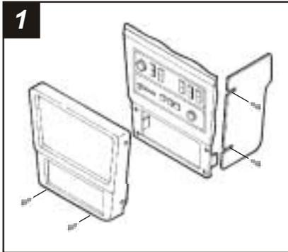
Disconnect the negative battery terminal to prevent an accidental short circuit. Remove (1) Phillips screw and (1) plastic twist-lock screw securing each side panel to the lower dash console. Remove (2) Phillips screws from the base of the radio trim bezel and remove the bezel. Remove (4) screws securing the factory pocket to the sub-dash and remove the pocket.
