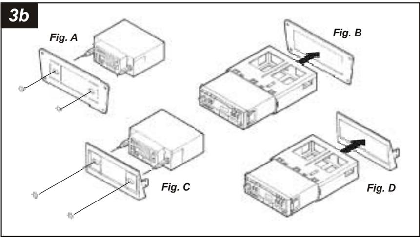
**200 SERIES (LOWER DASH), 100 SERIES:** For 2-Shaft head units, slide the aftermarket head unit into the **Radio Housing** and secure with shaft nuts. (see Fig. A). For DIN head units, cut and remove the shaft supports from the kit. Slide the DIN cage into the kit and secure by bending the metal locking tabs down. Slide the aftermarket head unit into the cage until secure. (see Fig. B)
