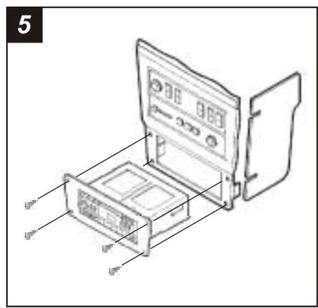
Re-connect the battery terminal and test the unit for proper operation. Mount the head unit/kit assembly to the sub-dash with those screws previously removed in step #1.
