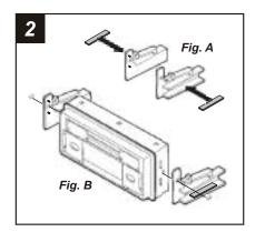
Peel away the paper backings from the *Tape Strips* and stick the Strips to the lower shelves of the *Mounting Clips*. (see Fig. A). Secure the *Mounting Clips* to the sides of the *Radio Housing* with (2) Carriage Bolts and (2) Keps Nuts supplied. (see Fig. B). Skip to the Installation Instructions for ALL VEHICLES on Page #2.
