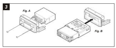
2-SHAFT HEAD UNITS: Slide the aftermarket head unit into the kit and secure with shaft nuts. (see Fig. A)
