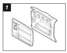
Disconnect the negative battery terminal to prevent an accidental short circuit. Unclip the plastic trim piece located below the steering column. Unclip the dash trim bezel. Pull the bezel over the steering column and disconnect the wiring. Using a flat-blade screwdriver, press down on the outside clips of the factory head unit and remove.
