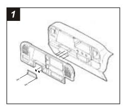
Disconnect the negative battery terminal to prevent an accidental short circuit. Remove the steering column filler panel and the ashtray. Unclip the dash trim bezel and remove. Using a small flat-blade screwdriver, press down on the outer clips of the factory head unit (or pocket). Disconnect the wiring and remove the unit.
