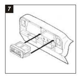
Re-connect the battery terminal and test the unit for proper operation. Slide the head unit/kit assembly into the sub-dash until the side clips engage.
