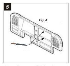
Using a file, remove 1/32" from the top and bottom edges of the dash trim bezel radio opening. (see Fig. A). Insert the head unit/kit assembly into opening (through the back of the bezel) to insure proper clearance has been established.
