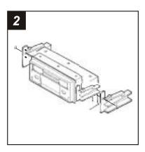
Secure the *Mounting Clips* to the sides of the *Radio Housing* with *(2) Carriage Bolts* and *(2) Keps Nuts* supplied. *Skip to the Installation Instructions for ALL VEHICLES on Page #2.*
