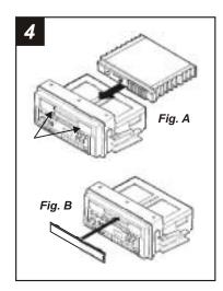
IF AN EQUALIZER WILL BE INCLUDED: Cut and remove the supports from the equalizer opening. Slide the aftermarket equalizer into the back of the Radio Housing. Using the hardware included with the equalizer, mount the unit to the kit. (see Fig. A) IF AN EQUALIZER WILL NOT BE INCLUDED: Snap the Equalizer Dummy Plate into the Radio Housing. (see Fig. B)
