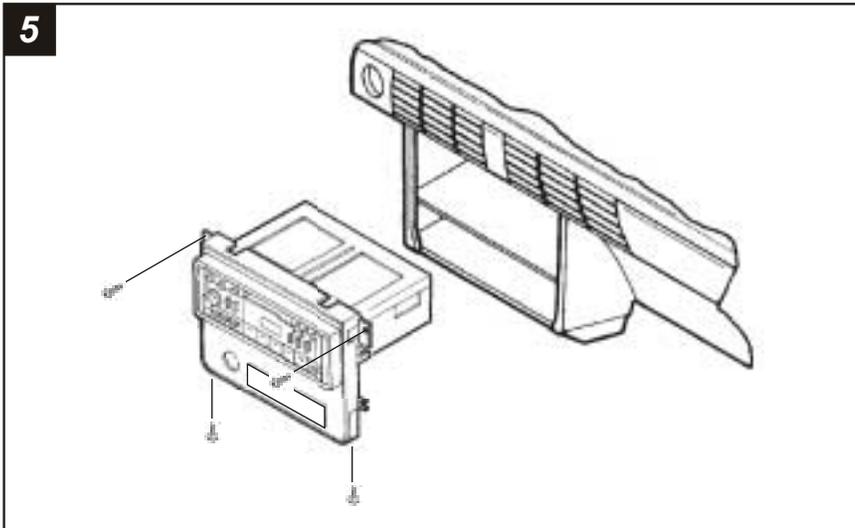
Re-connect the battery terminal and test the unit for proper operation. Mount the head unit/kit assembly to the sub-dash with (4) screws previously removed in step #1.
