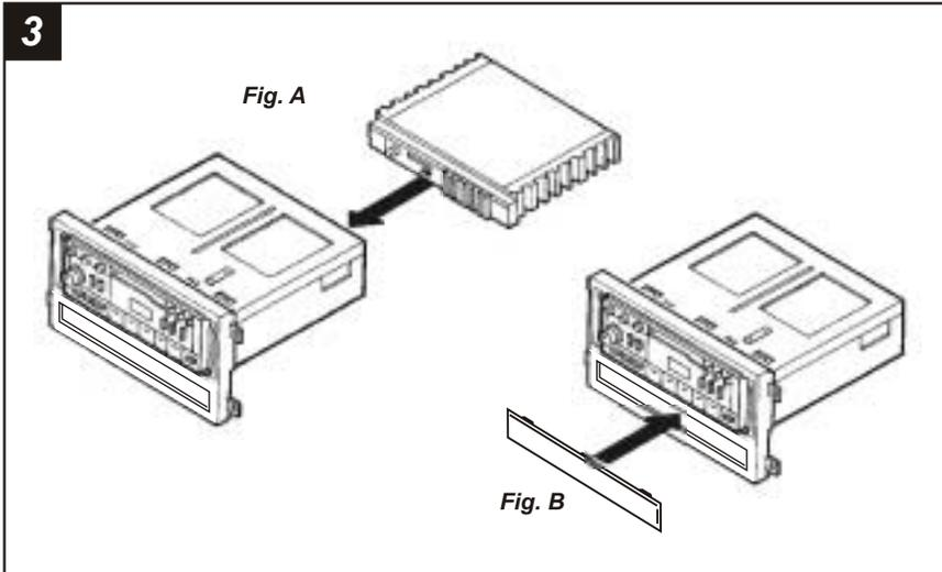
**IF AN EQUALIZER WILL BE INCLUDED:** Slide the aftermarket equalizer into the back of the **Radio Housing**. Using the hardware included with the equalizer, mount the unit to the kit. (see Fig. A)
