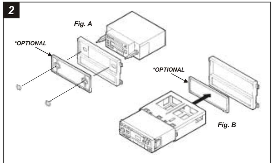
**2-SHAFT HEAD UNITS:** Slide the aftermarket head unit into the kit and secure with shaft nuts. (see Fig. A)
