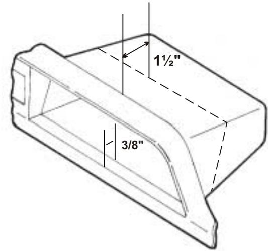
Using the dimensions above, cut and remove the rear portion of the factory pocket from the radio trim bezel.
