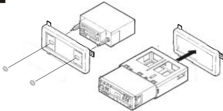
**2-SHAFT HEAD UNITS:** Slide the aftermarket head unit into the kit and secure with shaft nuts. (see Fig. A)
