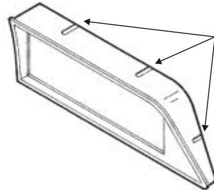
Locate the recessed slots on the top of the **Faceplate** and drill (1)  $3/16$ " hole into each slot.
