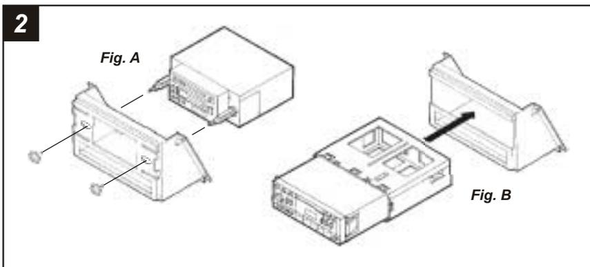
**2-SHAFT HEAD UNITS:** Slide the aftermarket head unit into the kit and secure with shaft nuts. (see Fig. A)
