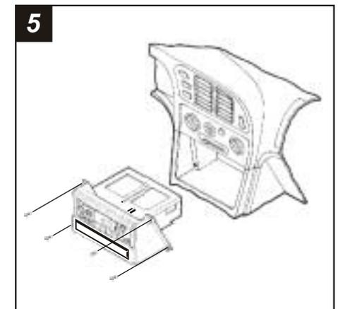
Re-connect the battery terminal and test the unit for proper operation. Mount the head unit/kit assembly to the sub-dash with (4) Phillips screws previously removed in step #1.
