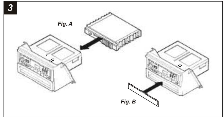
**IF AN EQUALIZER WILL BE INCLUDED:** Slide the aftermarket equalizer into the back of the **Radio Housing**. Using the hardware included with the equalizer, mount the unit to the kit. (see Fig. A)
