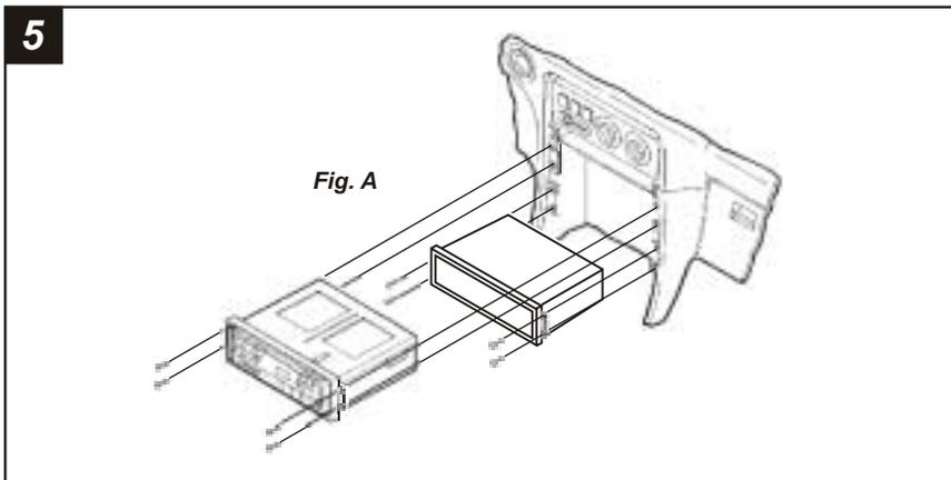
**ACCENT:** Re-connect the battery terminal and test the unit for proper operation. Mount the head unit/kit assembly to the sub-dash with (4) Phillips screws previously removed in step #1.
