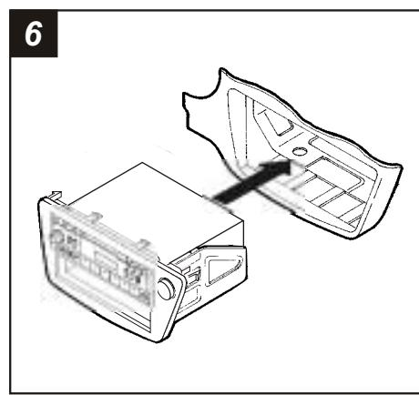
Locate the factory wiring harness in the dash. Metra recommends using the proper mating adaptor and making connections as shown. (Isolate and individually tape off the ends of any unused wires to prevent electrical short circuit).
