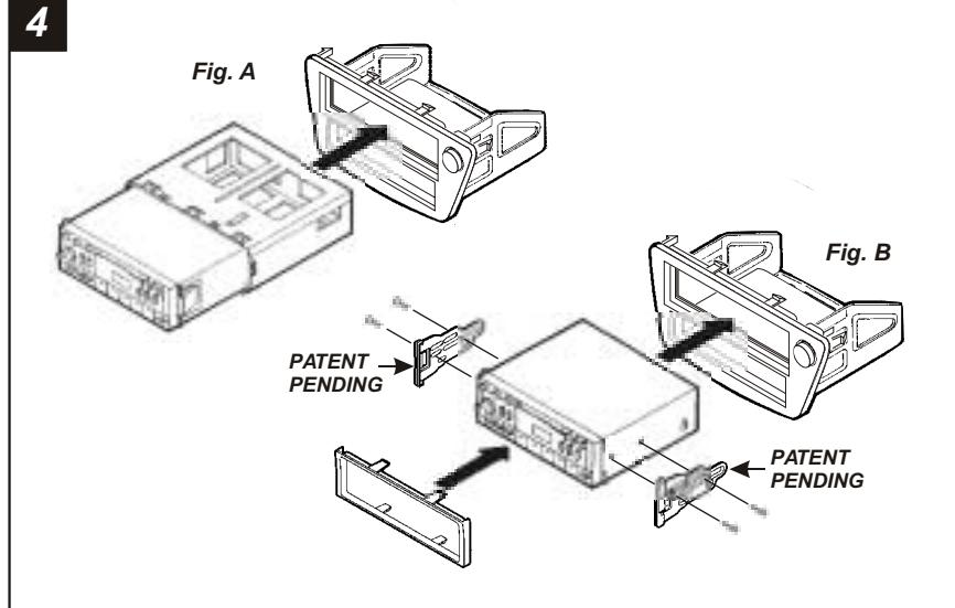
**DIN HEAD UNITS:** Slide the DIN cage into the kit and secure by bending the metal locking tabs down. Slide the aftermarket head unit into the cage until secure. (see Fig. A)
