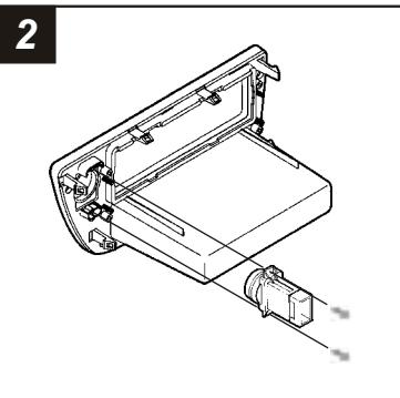
Mount the hazard switch to the back of the **Radio Housing** with (2) Phillips screws previously removed in step #1.
