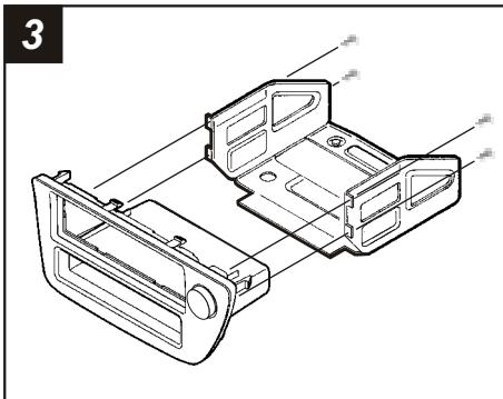
Mount the factory bracket assembly to the back of the **Radio Housing** with (4) Phillips screws previously removed in step #1.
