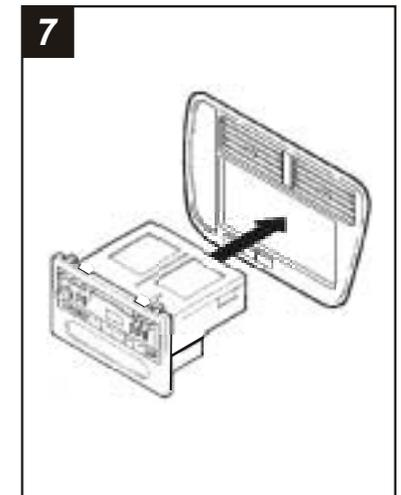
Snap the head unit/kit assembly into the radio trim bezel.
