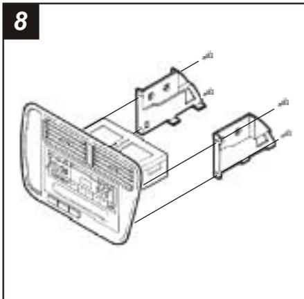
Mount the factory brackets to the back of the dash trim bezel with (4) Phillips screws previously removed in step #3.
