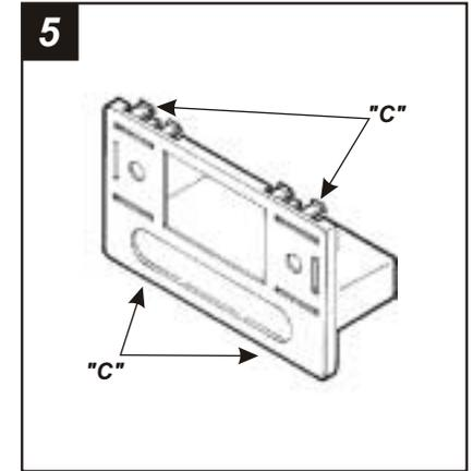
Cut and remove all mounting clips on the **Radio Housing** EXCEPT clips "C". The mounting clips can be identified by the stamped letter on each clip.
