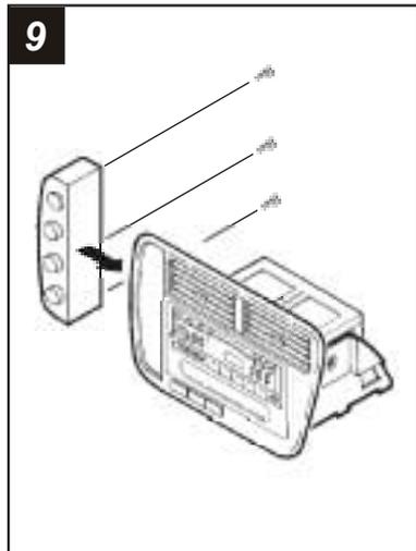
Mount the climate control pod to the dash trim bezel with (3) screws previously removed in step #2.
