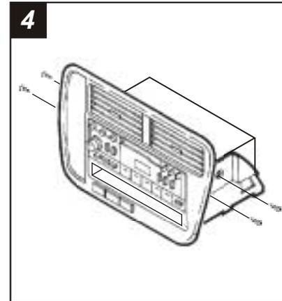
Remove (4) Phillips screws securing the factory brackets to the head unit assembly and slide the assembly out the front of the dash trim bezel.
