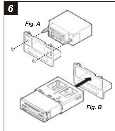
**2-SHAFT HEAD UNITS:** Slide the aftermarket head unit into the **Radio Housing** and secure with shaft nuts. (see Fig. A)
